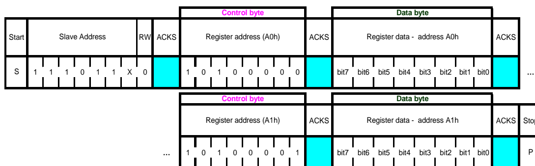
Figure 9: I 2 C multiple byte write (not auto-incremented)
